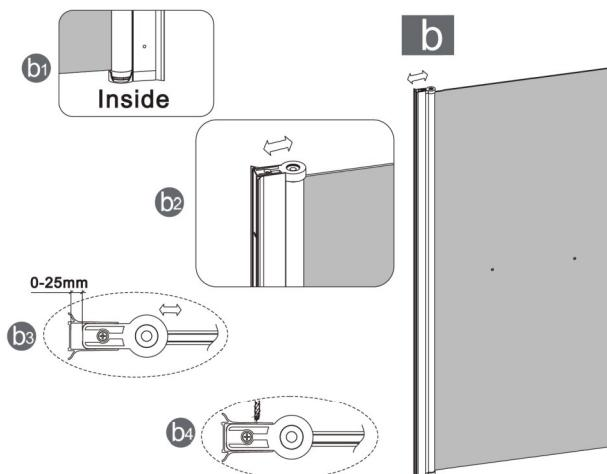
► Assemble the door with the vertical profile and the hinges as in the sketch. You can set up to 35mm.
