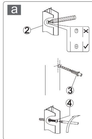
► Level and screw the vertical wall profiles.
